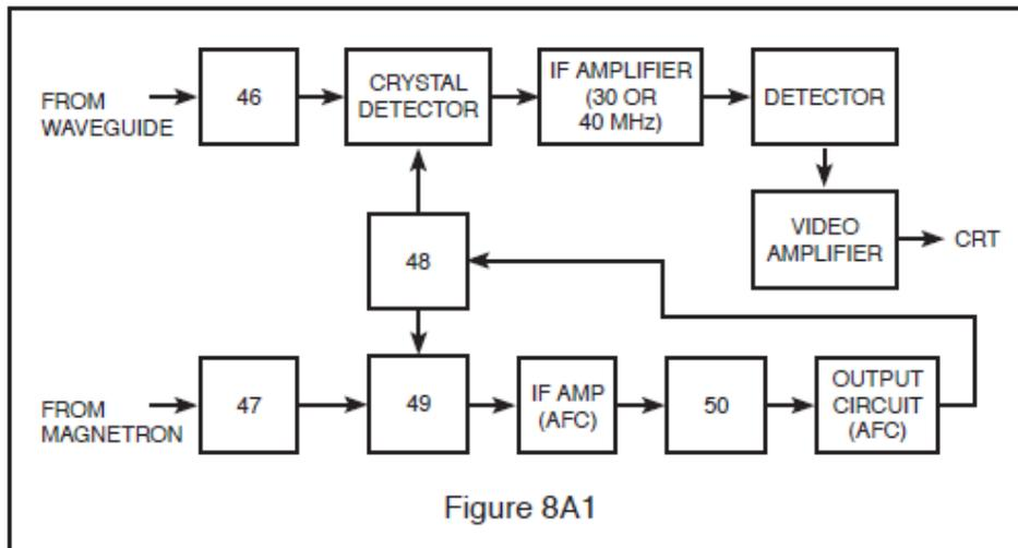
8-21C4 What device(s) could be used as the local oscillator in a RADAR receiver?
